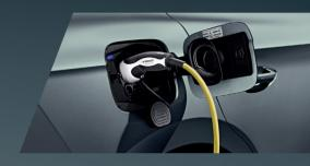
The iV Universal Charger is a portable AC charging solution that provides full flexibility for all types of AC charging. It comes with plugs for 220-V and 400-V sockets.
