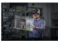
ŠKODA AUTO tests augmented reality glasses for production line maintenance and technical training The HoloLens consists of the actual glasses, which make holograms visible, and a camera-projector unit. The visor can be flipped up at any time to step out of the mixed reality.
