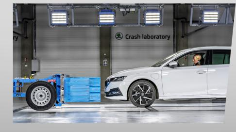
Nowadays, ŠKODA AUTO operates its own crash lab that enables two cars to be accelerated into each other at speeds of up to 65 km/h, or one vehicle at up to 120 km/h.
