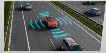
**Emergency Assist** If the driver becomes incapacitated, e.g. for health reasons, Emergency Assist brings the vehicle safely to a halt and activates the hazard warning lights. Emergency Assist is available for vehicles with DSG. Emergency Assist is not available for the FABIA, SCALA and KAMIQ model series.
