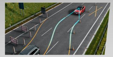
**Adaptive Lane Assist** uses the multifunction camera on the windscreen. It helps to keep the vehicle in lane by adjusting the steering whenever necessary. The system is also able to identify the edge of the road and temporary lane markings, for example, in road works.
