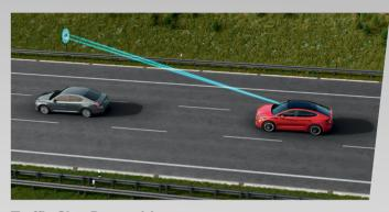
**Traffic Sign Recognition** For cars with a navigation system, this assistance system matches recognised traffic signs to data from the navigation system.
