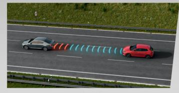
Adaptive Cruise Control (ACC) keeps the car at a constant safe distance from vehicles in front. For cars with DSG and the OCTAVIA also in combination with manual transmission, ACC includes Stop&Go, automatically adjusting the speed to the vehicle in front and braking to a standstill if necessary. The ACC's predictive function uses images from the windscreen camera and data from the navigation system to detect speed limits and bends and automatically adjust the speed.
