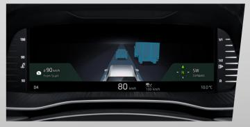
**The 3D display for assistance systems** shows objects around the vehicle captured by the multifunction camera in the Virtual Cockpit. Available for the OCTAVIA and ENYAQ iV.
