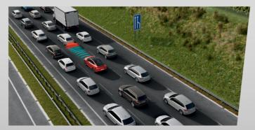
**Traffic Jam Assist** is available for vehicles with DSG and the OCTAVIA also in combination with manual transmission. The system automatically starts and brakes the car in heavy traffic.
