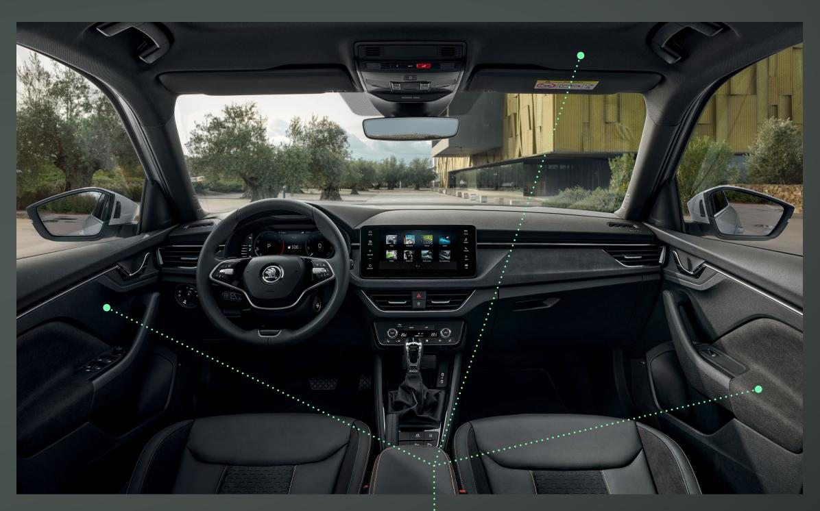
Wood flour, recycled materials, hemp and kenaf are used in the door panels and headliner
